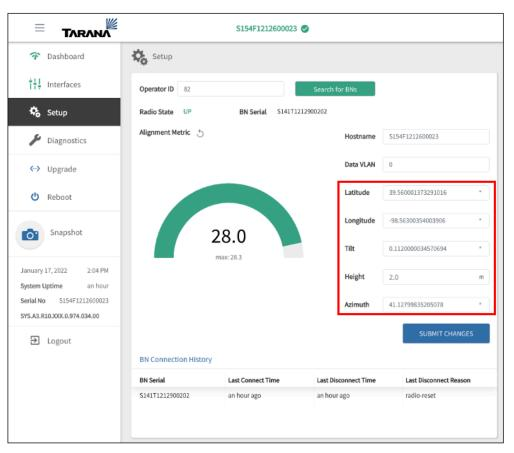
For CBRS models, after Submit Changes is clicked, an Installation Parameters pop-up will appear. Verify the installation parameters are correct, then enter your CPI ID and click Confirm.
