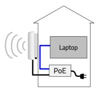
Step 2. Assign a static IP address of 192.168.10.10 to the laptop's Ethernet port.
