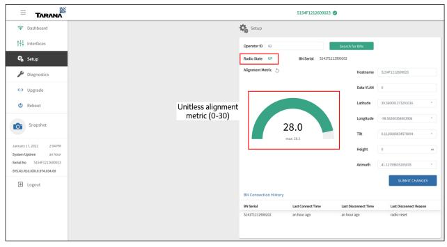
Figure 9: Radio State and Alignment Metric
