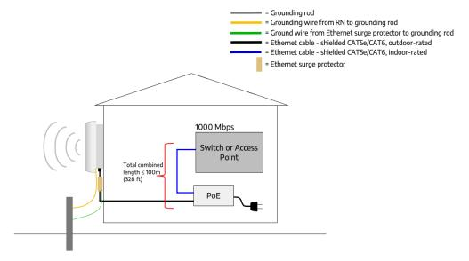
**Note:** Both electrical grounding and chassis ground are *always* required for G1 operation.
