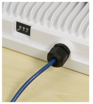
Properly terminate and test the Ethernet cable run before proceeding. This should include power verification on all pins of the Ethernet cable using a PoE tester.
