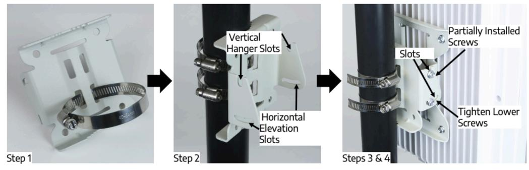
Figure 5: Elevation Bracket Installation (Pole Mount)
