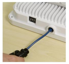
Step 5. Insert the cable into the RN Ethernet port and screw the cord grip body into the RN, taking care to not cross thread the plastic threads of the cord grip body with the aluminum threads of the RN enclosure.
