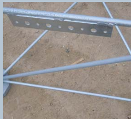
Integral transmission line supports
