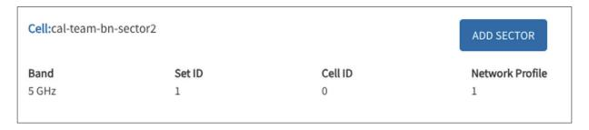
Figure 17: Cell definition within TCS allows the operator to configure set and cell IDs
