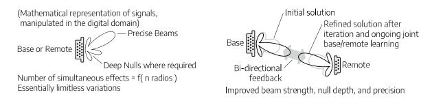
Figure 2: G1's precise digital beams and nulls enable greater signal strength and less interference
