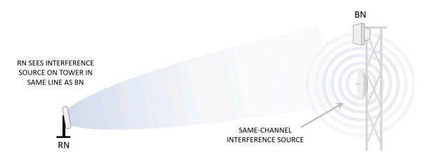
Figure 24: Co-linear interference at the tower impacts downlink performance
