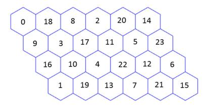
Figure 18: A set is a collection of 24 cells, each consisting of one to four sectors—each cell represents a geographic area of 9 km² (3 km by 3 km).
