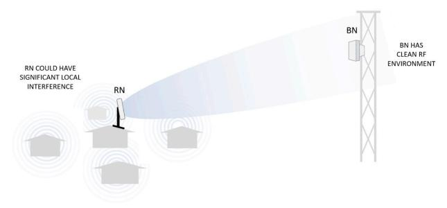
Figure 29: Remote node experiences significant local interference, impacting downlink performance
