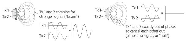
To control, adjust relative timing and power
