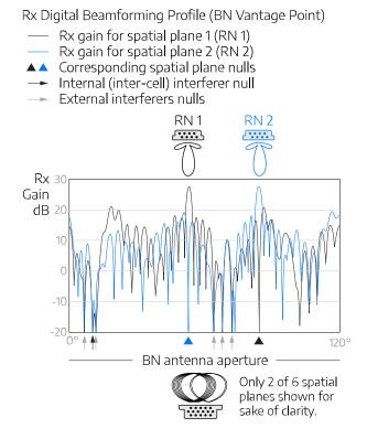
Figure 9: Deep nulling of unwanted signals (internal and external)
