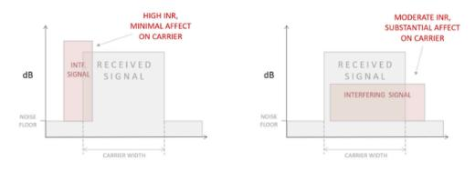
Figure 27: The impact of INR is a function of strength and width of interference
